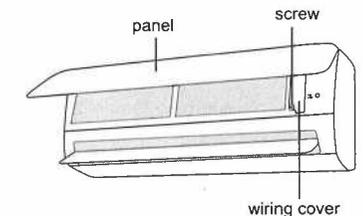
2. Make the power connection wire go through the cable-cross hole at the back of indoor unit and then pull it out from the front side.
