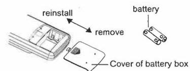
1. Press the back side of remote controller marked with "⊞", as shown in the fig, and then push out the cover of battery box along the arrow direction.
