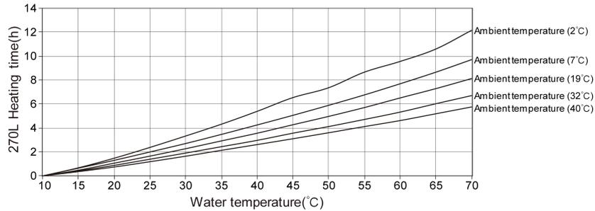
Fig. 4.8-2 GRS-2.3Pd/TD270ANpH-K heating time to different hot water target temperatures for different ambient temperatures (Only heat pump)
