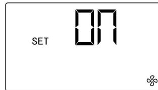
Fig.4.5-6 Ventilation function is on
