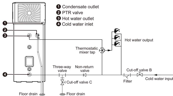
Fig.3.2-1 Unit Installation Diagram
