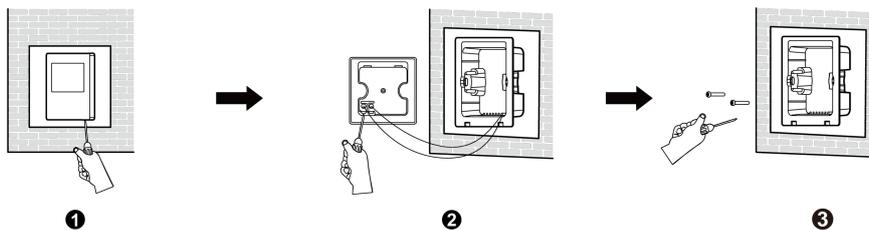
Fig.3.8-4 Removal of Wired Controller
