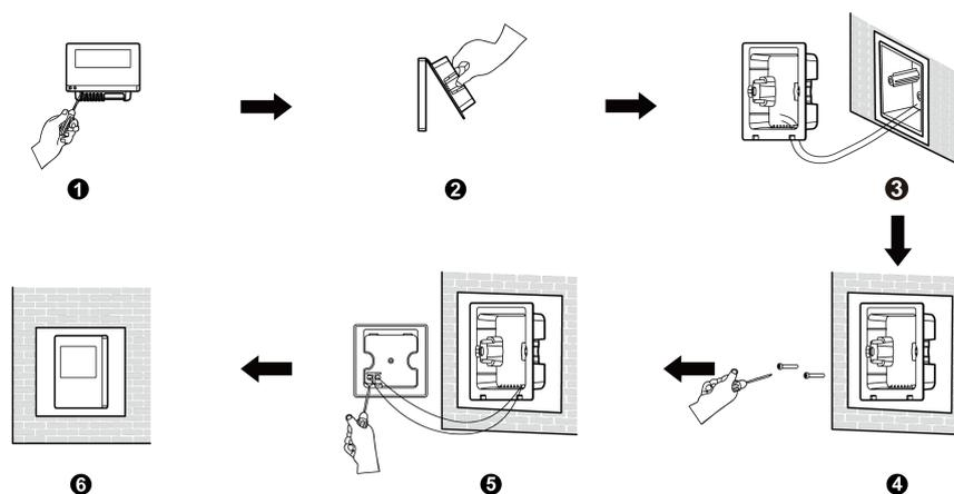
Fig.3.8-3 Installation of wired controller
