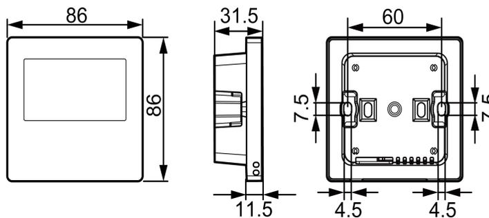
Fig.3.8-1 Dimensions of Wired Controller
