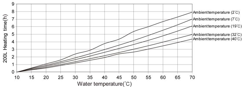
Fig. 4.8-3 GRS-2.3Pd/TD200ANpH-K heating time to different hot water target temperatures for different ambient temperatures (Only heat pump)
