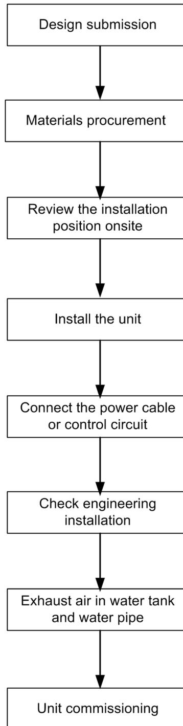
Fig.1-1 Flowchart for installing the unit
