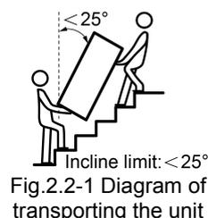
Fig.2.2-1 Diagram of transporting the unit
