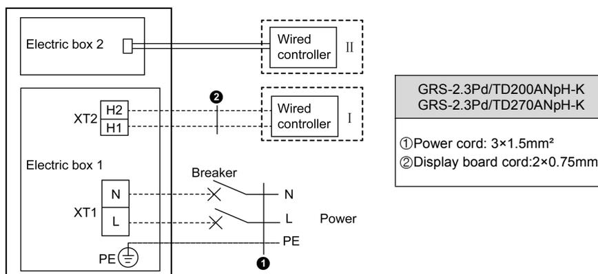
Fig.3.7-1 External wiring
